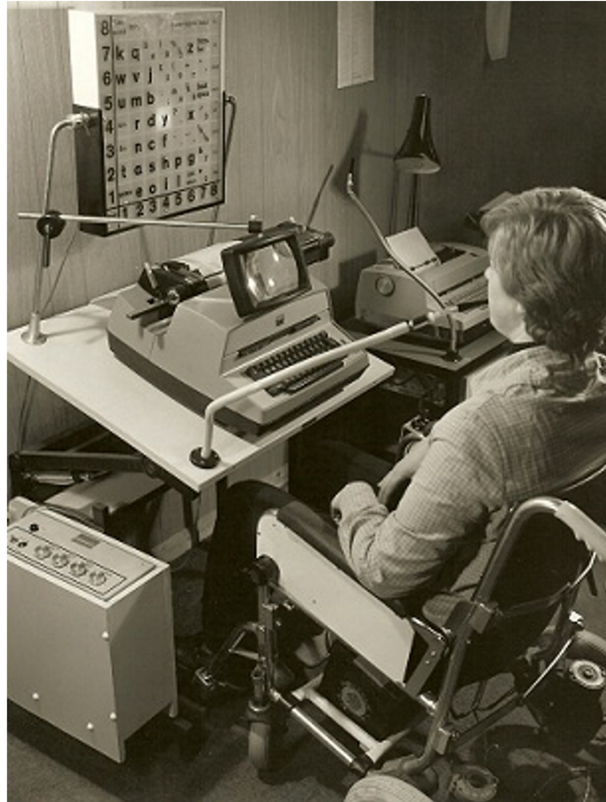
A person in a wheelchair operating an old computer using a desk-mounted sip and puff device called the POSSUM.
